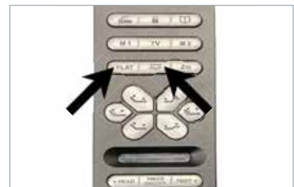
Method 1: Press the FLAT+ UNDER BED LIGHT buttons to reset the system.
